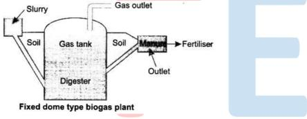
The biogas plant has a dome-like structure built with bricks. A slurry of cow-dung and water is made in the mixing tank from where it is fed into the digester. The digester is a sealed chamber in which there is no oxygen.
