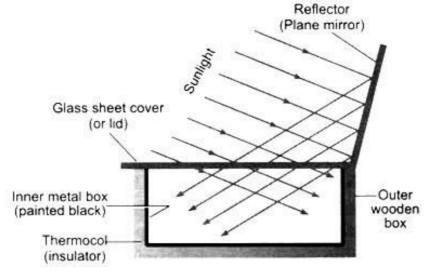
Construction of a box-type solar cooker:
