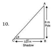
Let the Sun's elevation be  $\theta$ Length of pole = 6 m, length of shadow =  $2\sqrt{3}$ m From  $\triangle ABC$ ,  $\frac{AB}{BC} = \tan \theta$  (using Pythagoras theorem)  $\Rightarrow \quad \frac{6}{2\sqrt{3}} = \tan \theta$   $\Rightarrow \quad \tan \theta = \frac{3}{\sqrt{3}} = \sqrt{3} = \tan 60^{\circ}$   $\Rightarrow \quad \theta = 60^{\circ}$ Hence sun's elevation is 60°
