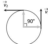
$= 2(r\omega) \sin(90^\circ / 2) = 2 \times 1 \times \frac{2\pi}{T} \times \frac{1}{\sqrt{2}}$ $= \frac{4\pi}{60\sqrt{2}} = \frac{\pi\sqrt{2}}{30} \frac{\text{cm}}{\text{sec}} \quad [\text{As } T = 60 \text{ sec}]$ |
