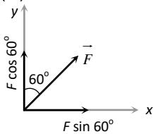
The component of force in vertical direction
