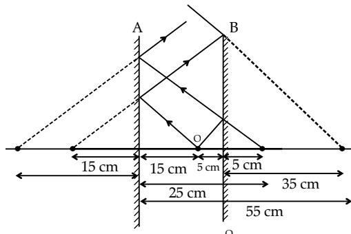
From ray diagram no image is formed at 45 cm.
