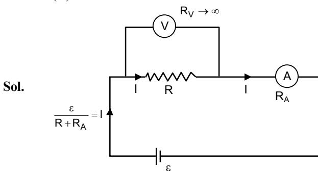
$$\text{Reading of ammeter } I = \frac{\epsilon}{R+R_A}$$
