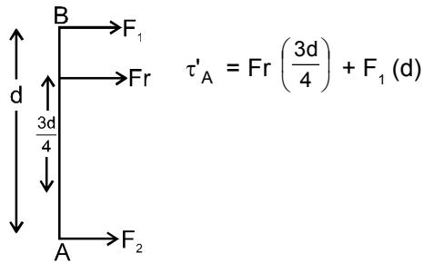
$$(F_1 + F_2) \frac{d}{2} + F_2 d = (F_1 + F_2) \left(\frac{3d}{4}\right) + F_1 d$$
