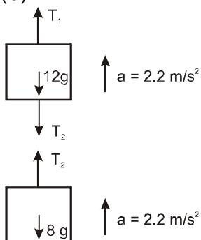
$$T_2 - 8g = 8a \text{ [Newton's II law for } 8\text{ kg block]}$$
