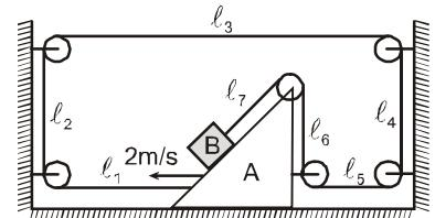
$l_2, l_3, l_4, l_6$  are remain constant.  $l_1 + l_5 =$  constant so,  $l_7$  will also be constant, so, only velocity of B is along horizontal = 2 m/s.
