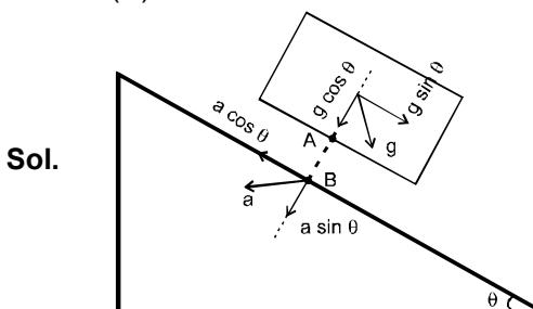
acceleration of point A and B must be some along the line ⊥ to the surface
