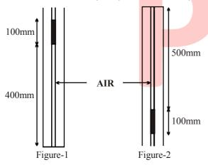
The tubing is now inverted, figure-2, and the air column is seen to increase in length to 500 mm. Use this observation to calculate a value for atmospheric pressure, expressed in
