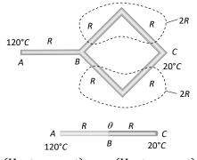
$(\text{Heat current})_{AC} = (\text{Heat current})_{AB}$  $\frac{(120-20)}{2R} = \frac{(120-\theta)}{R} \Rightarrow \theta = 70^{\circ}\text{C}$
