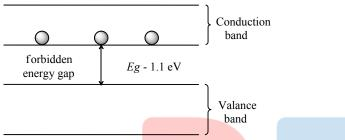
In semiconductors, valence band and conduction band are separated by an energy gap called the forbidden energy gap. It is very small. At room temperature some electrons in valence band acquire thermal energy. This energy is more than forbidden energy gap  $E_g$ , thus they jump into the conduction band and leaves their vacancy in the valence band which act as holes. Hence, at room temperature valence band is partially empty and conduction band is partially filled.
