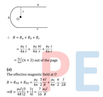
As per Fleming's Right Hand rule, direction of magnetic field is perpendicular and in the plane of paper
