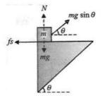
$mg\sin\theta$  is the pseudo force on m $N + mg\sin\theta + \sin\theta = mg$  or  $N = mg\cos^2\theta$ And for no slipping,  $mg\sin\theta\cos\theta \ge \mu N$  $mg\sin\theta\cos\theta \le \mu mg\cos^2\theta$  or  $\mu \ge \tan\theta$
