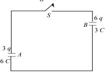
Let  $q_1$  and  $q_2$  be the charge after switch *S* has been closed.
