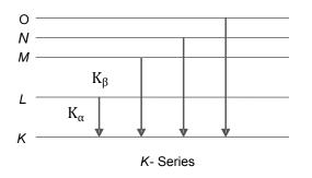
$\therefore$   $K_{\alpha}$  and  $K_{\beta}$  X-rays are emitted when there is transition of electron between the levels n=2 to n=1 and n=3 to n=1 respectively.
