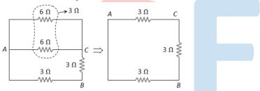
So the equivalent resistance between points *A* and *B* is equal to
