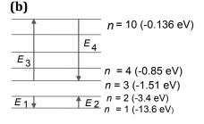
$E_1 = -13.6 - (-3.4) = -10.2 \text{ eV}$   $E_2 = -3.4 - (-13.6) = +10.2 \text{ eV}$   $E_3 = -0.136 - (-1.51) = -1.374 \text{ eV}$  $E_4 = -1.51 - (-0.136) = -1.374 \text{ eV}$
