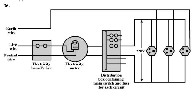
A fuse in a circuit prevents damage to the appliances and the circuit due to overloading. Otherwise, the appliances or the circuit may be damaged.
