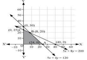
The corner points are A (24, 0), B (8, 20), and C (0, 25). The values of Z at these corner points are as follows:
