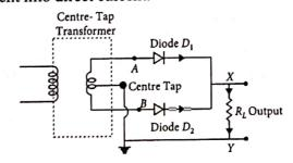
A full wave rectifier consists of two diodes connected in parallel across the ends of secondary winding of a center tapped step down transformer. The load resistance  $R_L$  is connected across secondary winding and the diodes between A and B as shown in the circuit.
