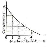
this means  $t_{1/2}$  is independent of initial concentration. Figure shows that typical variation of concentration of reactant exhibiting first order kinetics. It may be noted that though the major portion of the first order kinetics may be over in a finite time, but the reaction will never cease as the concentration of reactant will be zero only at infinite time.
