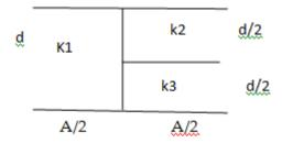
You are given an air filled parallel plate capacitor C1. The space between its plates is now filled with slabs of dielectric constants K1 and K2 as shown in C2. Find the capacitances of the capacitor C2 if area of the plates is A and distance between the plates is d.
