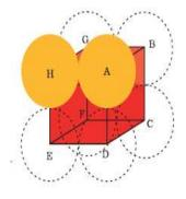
In a simple cubic lattice the atoms are located only on the corners of the cube. The particles touch each other along the edge (Fig. 1.22). Thus, the edge length or side of the cube 'a', and the radius of each particle, r are related as
